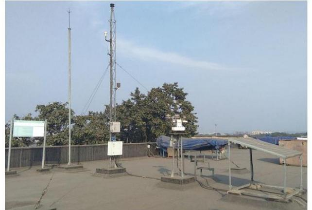
Fig. 8 Photograph of digital pyranometer system
