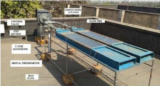
Fig. 2 Photograph of test-rig
